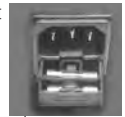
Fuse compartment and spare fuse are located below detachable power cord receptacle
