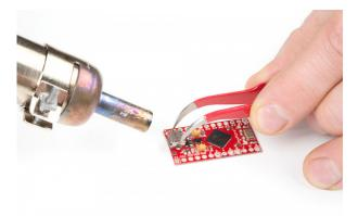
A micro-B connector being removed from a Pro Micro for a Tech Prank. Be sure to rework the board on a heat resistant material!
