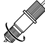
**4** (1) Loosen the tool securing screw on the tool carriage.
